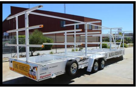
Ausco Products has designed and manufactured a number of state of the art and durable rowing boat trailers that are capable of long distance journeys across the country, to weekly regattas around WA. The Ausco trailer consists of a strong and durable galvanised RHS frame, large retractable side steps and folding down supports to make boat loading much safer, quicker and easier.
