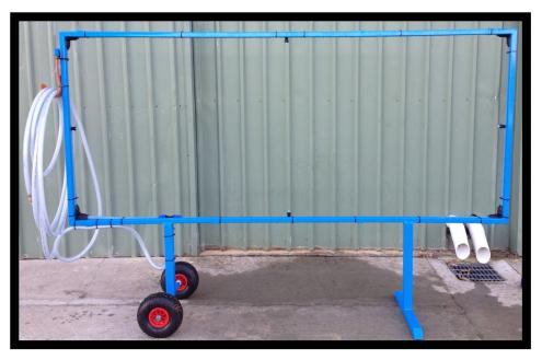
Ausco Products has designed and manufactured a boat washing system that significantly decrease the amount of pack up time for clubs and schools. The system is designed such that the boat passes through the middle of the spray jets as it is walked inside the shed. There are four main jets that run off mains pressure to wash the top, bottom and inside the hull as it passes through.
