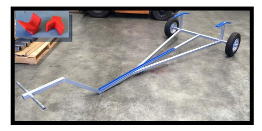
Ausco Products has designed and manufactured a quality and durable safety boat trailer that will outlast any other trailer on the market. The Ausco trailer consists of a strong and durable galvanised frame, with alloy wheels and proper trailer wheel bearings to suit the salty environment. The Trailer is customisable to meet your requirements, whether size or boat runner type.
