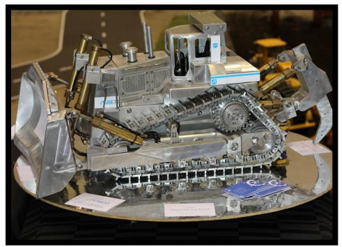
Ausco Products are proud to announce the design and produce of a 1:15 scale, full hydraulic radio controlled Bulldozer. The hydraulic function is controlled via 4 valves for replication of a real machine when operating the blade and ripper functions.
